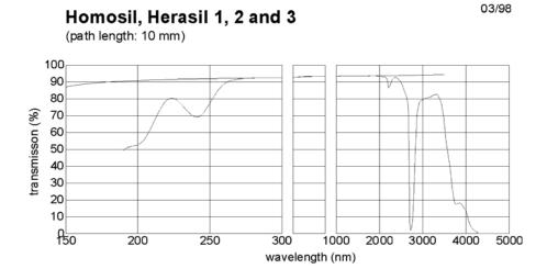
Typical spectral transmission including Fresnel reflection loss. The uppermost nearly straight line indicates the calculated Fresnel reflection loss of two uncoated surfaces.
