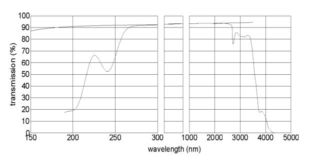
Typical spectral transmission including Fresnel reflection loss. The uppermost nearly straight line indicates the calculated Fresnel reflection loss of two uncoated surfaces.
