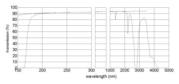
Typical spectral transmission including Fresnel reflection loss. The uppermost nearly straight line indicates the calculated Fresnel reflection loss of two uncoated surfaces.
